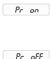
Enables the Auto Power Off function. The power will be turned off after 2 minutes if a key has not been pressed for 2 minutes and the scale is at zero. If there is any weight on the scale or a key is pressed, the scale will continue to work.
